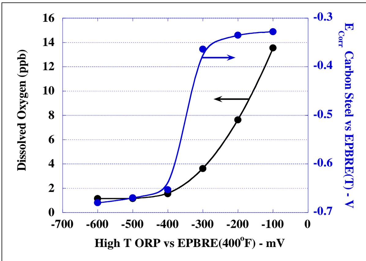
*In this case notice how the corrosion potential of carbon steel declines as oxygen is removed from the system with the oxygen scavenger erythorbic acid. The data is plotted with the @T ORP data at 400F.*
