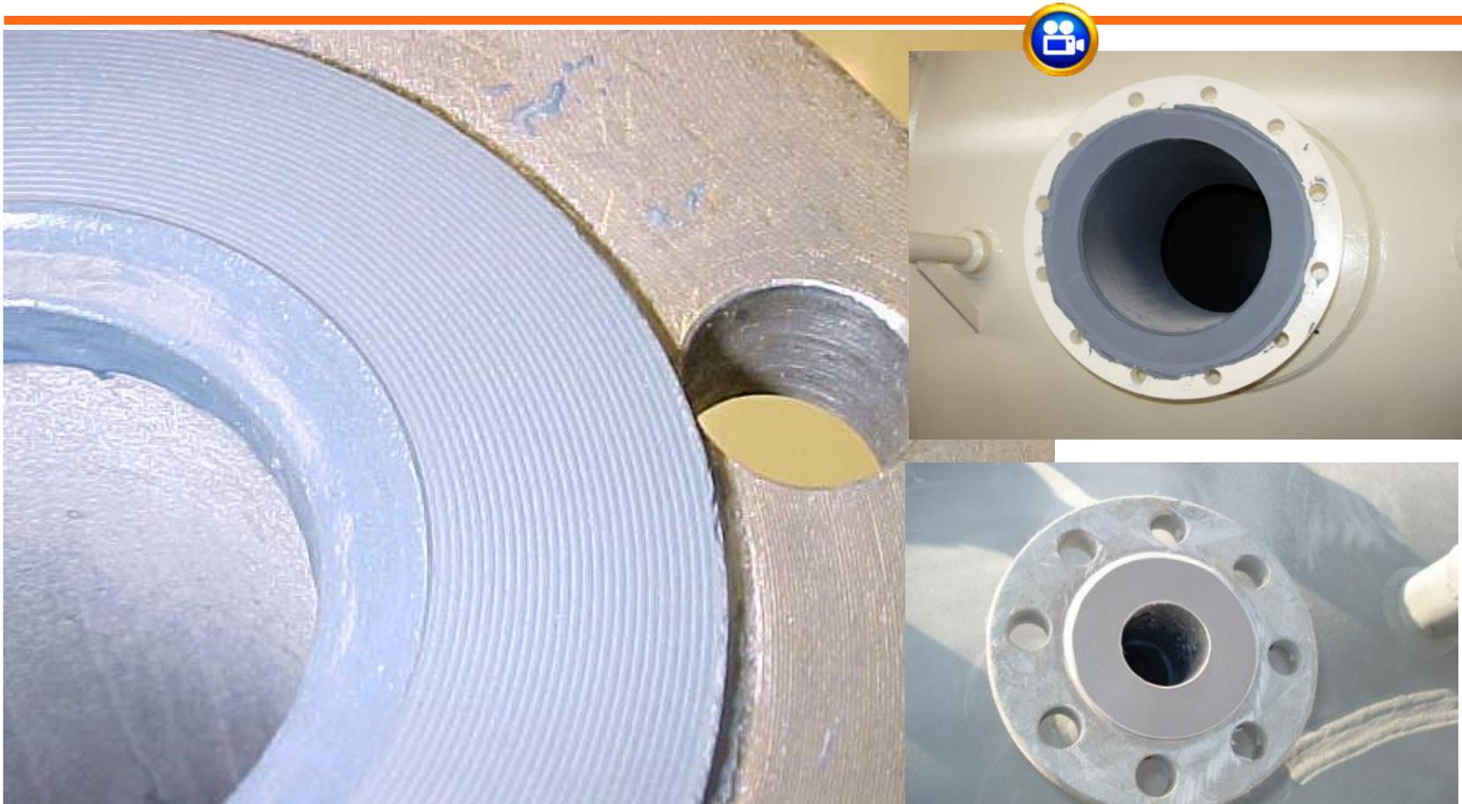
Flange faces formed using Belzona materials to prevent corrosion and leaks
