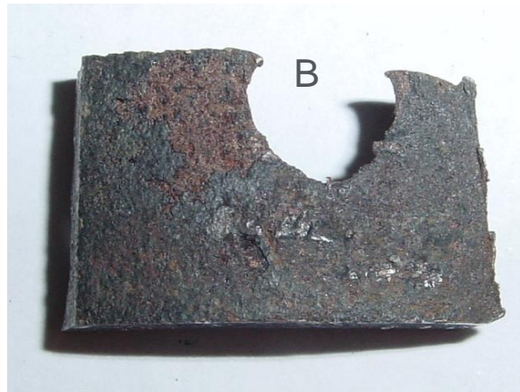
Figure 2: Photographs showing through thickness hole on ID (A) and OD (B) after mechanical removal of hard tubercle. Note conical crater of hole on ID.
