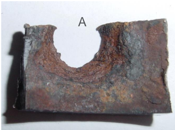
Figure 2: Photographs showing through thickness hole on ID (A) and OD (B) after mechanical removal of hard tubercle. Note conical crater of hole on ID.
