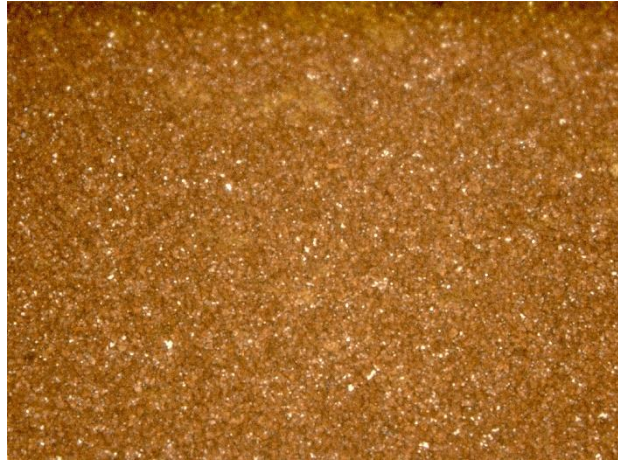
Figure 3: ID sound surface showing the presence of uniform brownish layer with incorporated numerous bright particles.
