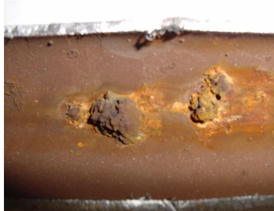
Figure 1: Close-up photos of split tube showing separate big (10 mm in height & diameters up to 12 mm) tubercles developed on ID surface exposed to hot gas.
