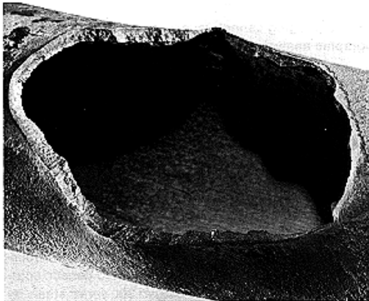
Figure 4. Typical window failure caused by hydrogen embrittlement
