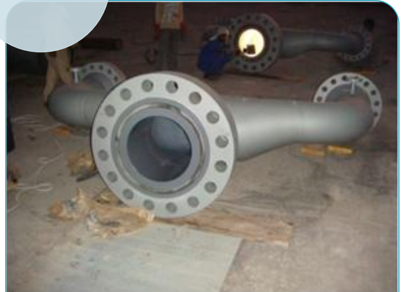
Surface protective coating against Erosion & Corrosion Pipes for Sea Water
