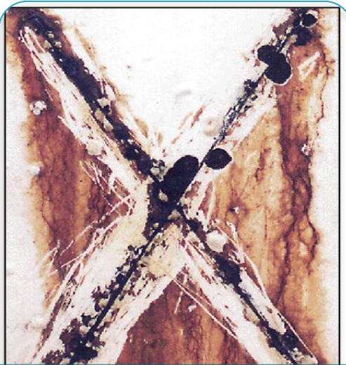
SC Epoxy - Two Coats (56% solids by volume)
